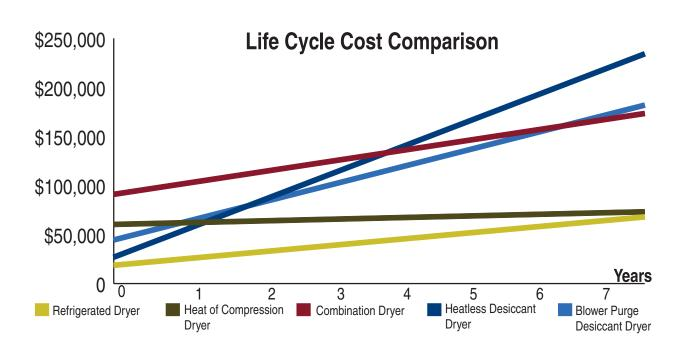
Based on 8760 hours of operation, maximum ambient temperature 100°F, air pressure at dryer inlet 100 psig, maximum air temperature at dryer inlet 100°F, maximum air flow rate of 1000 scfm, and \$0.10/kWh.
