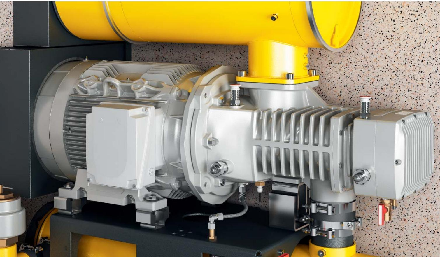
In DBS series blowers, power is transferred from the motor to the blower airend via an integrated gear drive. Following detailed testing in Kaeser's Research and Development Centers, this was found to be the most effective transmission solution for the speeds in this power size and machine class with regards to efficiency, dependability, and durability.
